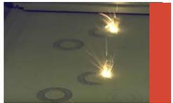
DMLS Direct Metal Laser Sintering
